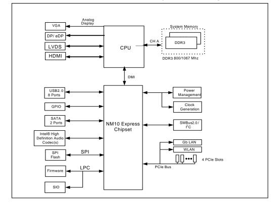
Figure 1-1. Intel® Atom<sup>™</sup> D2000 series/N2000 series System Block Diagram
